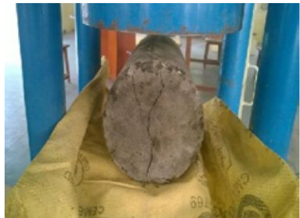
Fig. 2 Testing of cylinder for split tensile strength
